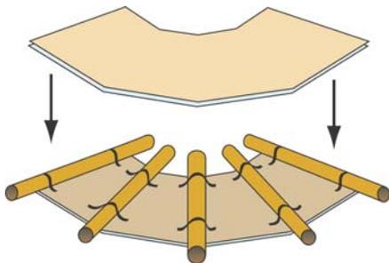
Top the tubes with the other piece of cardboard, so you have a "tube sandwich." Tape the two pieces of together cardboard at a few places around the edges.
