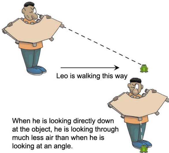
Notice that when you look through either of the topmost tubes (looking ahead or behind as you pass over the object), you are looking through more air than when you are looking straight down through the middle tube. Although in our demonstration there isn't enough of a difference in viewing pathlength to change the appearance of the object, if the air were foggy or smoky and you were a lot higher up in the sky, this angle would make quite a difference in how well you would see the ground.
