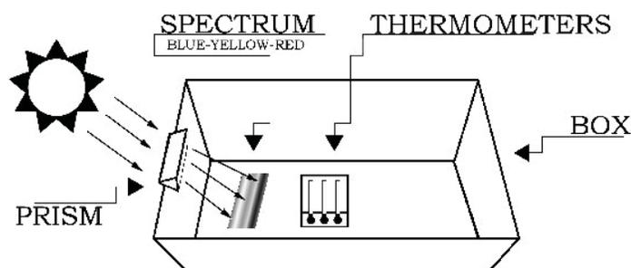
Figure 2. Initial setup for Herschel experiment with thermometers taped together and lined up.
