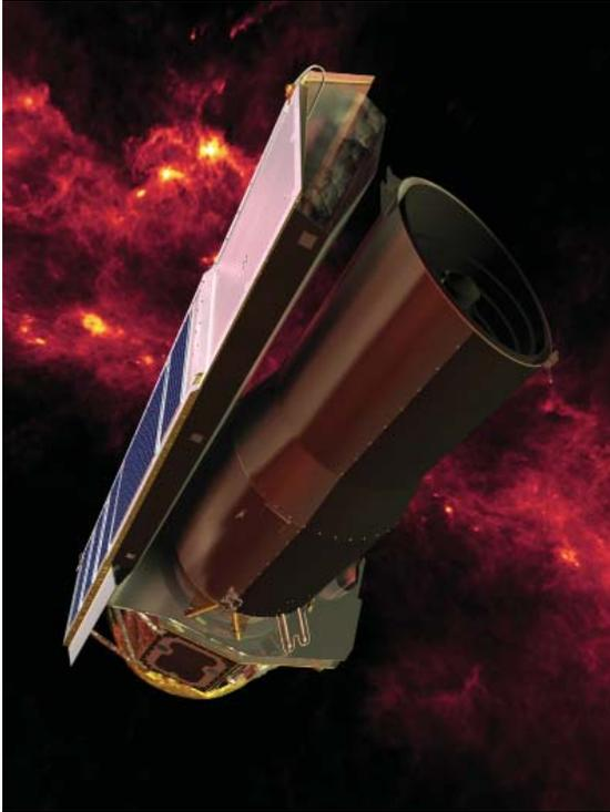
The Spitzer Space Telescope was launched into space by a Delta rocket from Cape Canaveral, Florida, on August 25, 2003. Spitzer's mission is to obtain images and spectra by detecting the infrared energy, or heat, radiated by objects in space between wavelengths of 3 and 160 microns (1 micron is one-millionth of a meter).
