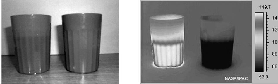
Above is a visible-light picture (left) and an infrared picture (right) of two cups. One cup contains cold water, while the other contains hot water. In the visible light picture we cannot tell which cup is holding cold water and which is holding hot water. In the infrared image, we can clearly "see" the glow from the hot water in the cup to the left and the dark, colder water in the cup to the right. If we had infrared eyes, we could tell if an object was hot or cold without having to touch it.
